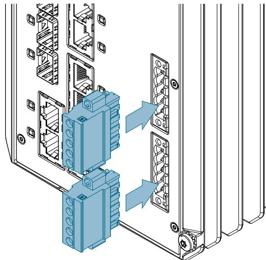
Figure 2.8 Assembling the Power Terminal Blocks
