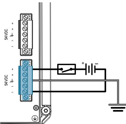
Figure 2.10 Single DC Power Input Configuration
