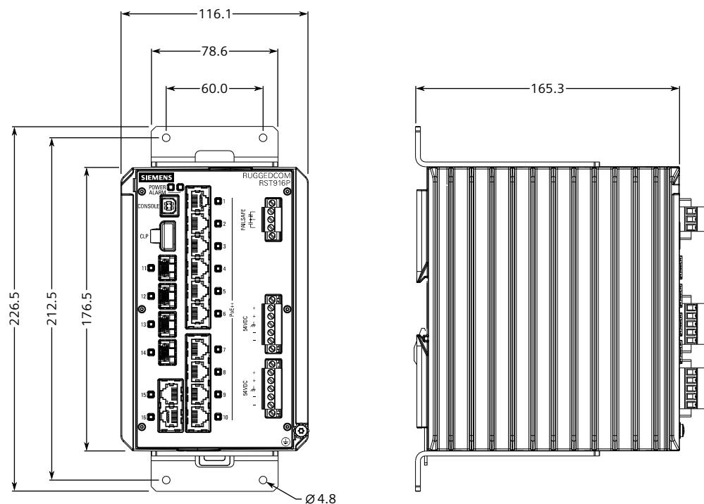
Figure 5.2 Panel Mount Dimensions (Rear Mount Orientation)
