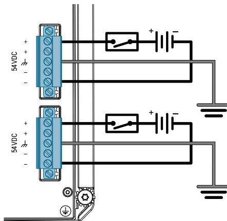
Figure 2.11 Dual DC Power Input Configuration
