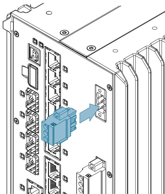
Figure 2.6 Assembling the Failsafe Alarm Relay Terminal Block
